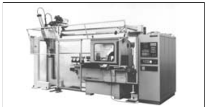
Fig. 9: Fässler D-250-C with automatic loading and unloading [4]
